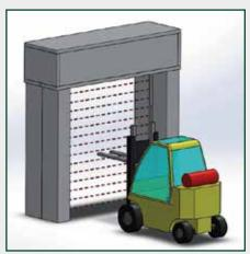
has four safety light barriers to minimise the risk of collisions and to enable contactless reversing of the rapid action door.
